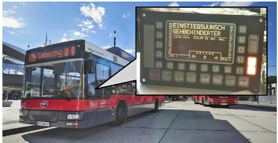
Figure 2: Bus driver display showing entry wish of wheel chair user at next station
